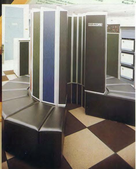
The speed of the CRAY-1 is partly attributable to the tightly packed circuits arranged in a semi-circle to minimize the distance between the computer's parts. The CRAY-1 is so fast that if the electricity had to travel too far, the computer would have to wait for it. The "seat" houses the equipment that supplies power to the rack of circuitry above it. A pump circulates Freon (the liquid used in air conditioners) through the cast aluminum racks to keep the computer cool.
