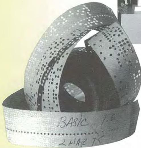
Bill Gates' Teletype tape to input the BASIC interpreter for the Altair was added to the collection. This BASIC interpreter became a *de facto* standard for microcomputers.
