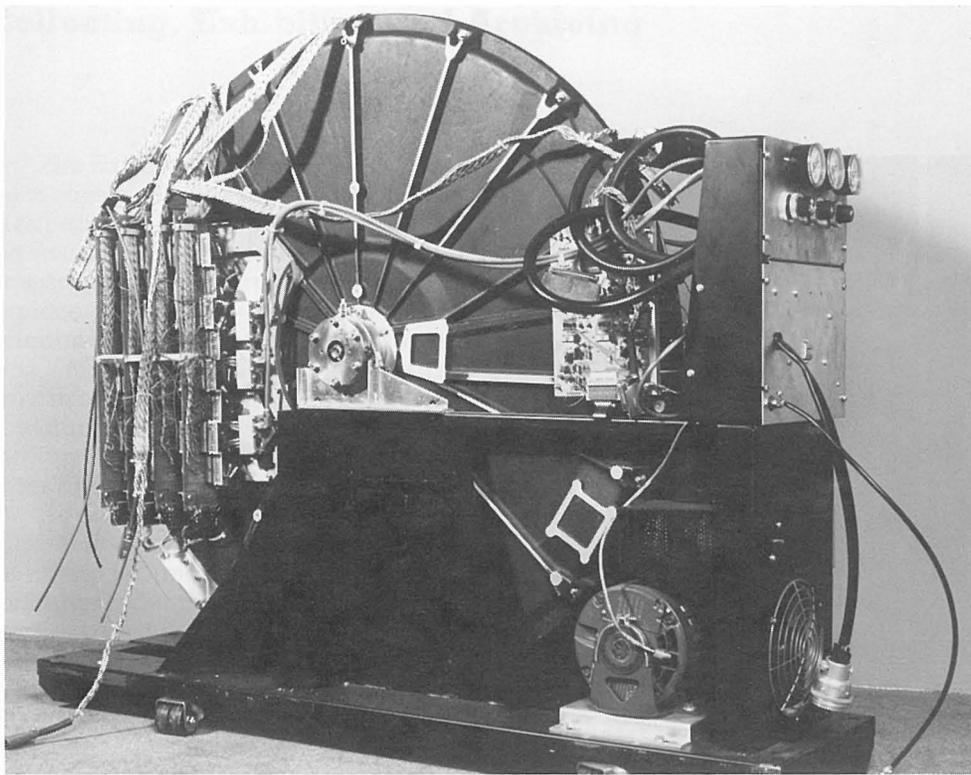
*This Burroughs Disk exhibited at The Computer Museum is only one of the thirteen synchronously rotating fixed head disks that comprised the 16M word main memory of Illiac IV.*
