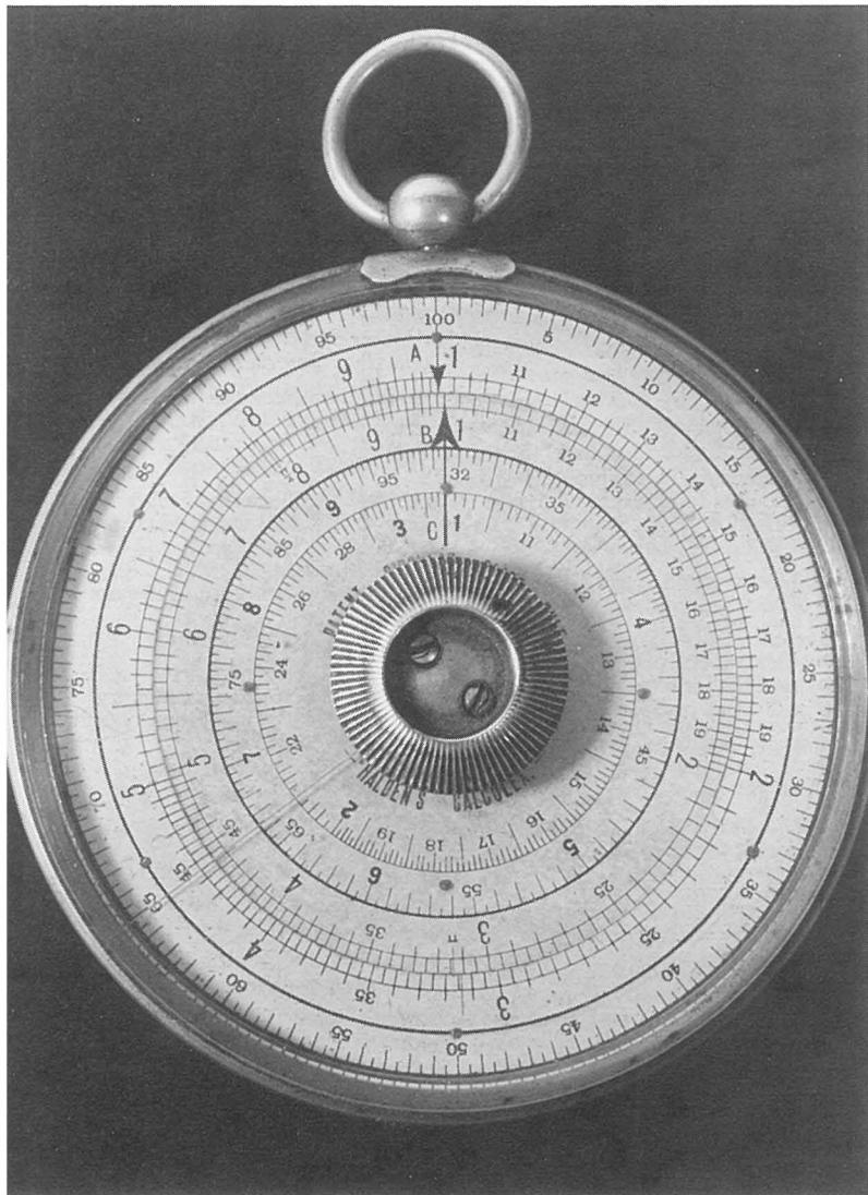
Manufactured by J. Halden and Company, London, during the 1920's, the pocket watch style calculator and slide rule has two logarithmic scales, A and B, on one side for multiplication, division and proportion which correspond to the A and B scales of an ordinary slide rule. Around the outer edge is a scale of logarithms read by a cursor. The inner circles contain a scale of square roots. The other side of the Calculex contains A and B scales for inverse proportions. Gift of Thomas McIntyre.
