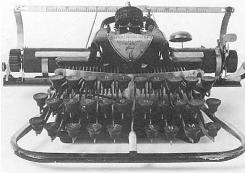
The "Blick" was the first typewriter intended to be readily portable. Designed and patented by George Blickensderfer in 1890, it was first sold in 1893. Each key had three positions, upper and lower case and a figure that positioned three levels of the printing wheel. Gift of Clark Prestia.
