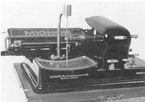
The Mignon typewriter is an indicator-type of machine, employing a stylus and a printed character table to manipulate the machine. Manufactured in Germany in 1908, the Mignon's advantage was its interchangeable letter table and type wheel, allowing typing in different languages. The Mignon is one of a gift of twenty-two typewriters from Clark Prestia. The donation represents an important part of the history of transducer equipment.
