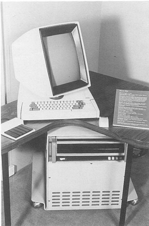
The Alto was designed in 1973 by Xerox Palo Alto Research Center as an experiment in personal computing with the goal of providing sufficient computing power, local storage, and input-output capability to satisfy the computational needs of a single user. The Alto significantly changed the office computing environment through its interactive nature and communication applications, such as electronic mail. On loan from Xerox PARC.
