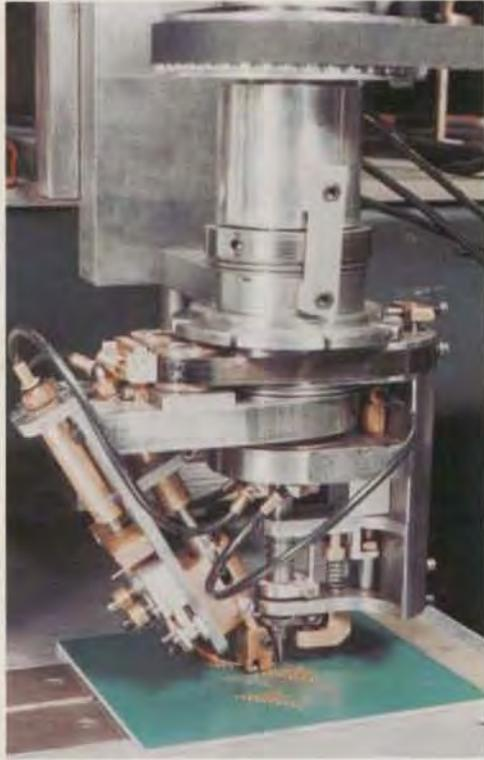
While driving home from work one evening in the fall of 1966, R. Page Burr (now a senior scientific officer at Kollmorgen Corporation) envisioned a way to improve interconnections on printed circuit boards. Connections were originally made by hand placing and soldering discrete wires. Mr. Burr's improvement consisted of copper lined holes interconnected by insulated wires. Interconnection devices of almost any complexity could be made because the insulated wires would be able to cross.
