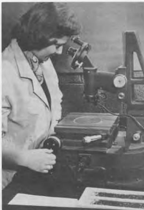
**Dimensional Check.** The machine die and the weight of the pressed cores had to be continually monitored to insure maximum uniformity of core size. Before each press run a dimensional check was made with a tool-maker's microscope in order to assure quality control.
