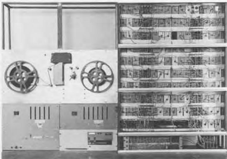
Constructed in 1966 as an unsponsored educational project of the Departments of Mathematics and Electrical Engineering at the University of California, Berkeley, the Delay Line Number Sieve performed 1 million tests per second. Navy surplus delay lines store the acceptable remainders for each modulus and circulate them synchronously. The machine has an idle mode in which all of the delay lines are connected in series and the data recirculated, so that the machine may be "stopped" and loaded.
