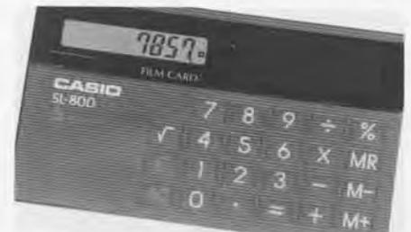
The SL-800 Film-Card announced by Casio in 1983 was the first calculator to be truly the size of a credit card. It sold for less than \$20. The SL-800 contains no moving parts. A fully automated factory produces an SL-800 in only 2.8 seconds. Gift of Casio Incorporated.
