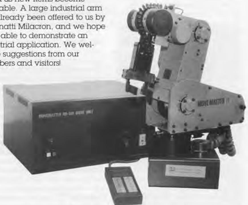
The Mitsubishi Movemaster uses its five joints and a gripper to pick up letter blocks and arrange them to spell a word typed in by the visitor. The arm is normally used for assembly or for handling chemicals.
