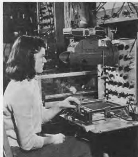
**Final Test.** The cores in the plane were then given a final pulse-response test in order insure their acceptability. If damaged, removal of defective cores from a plane was easy at this stage.
