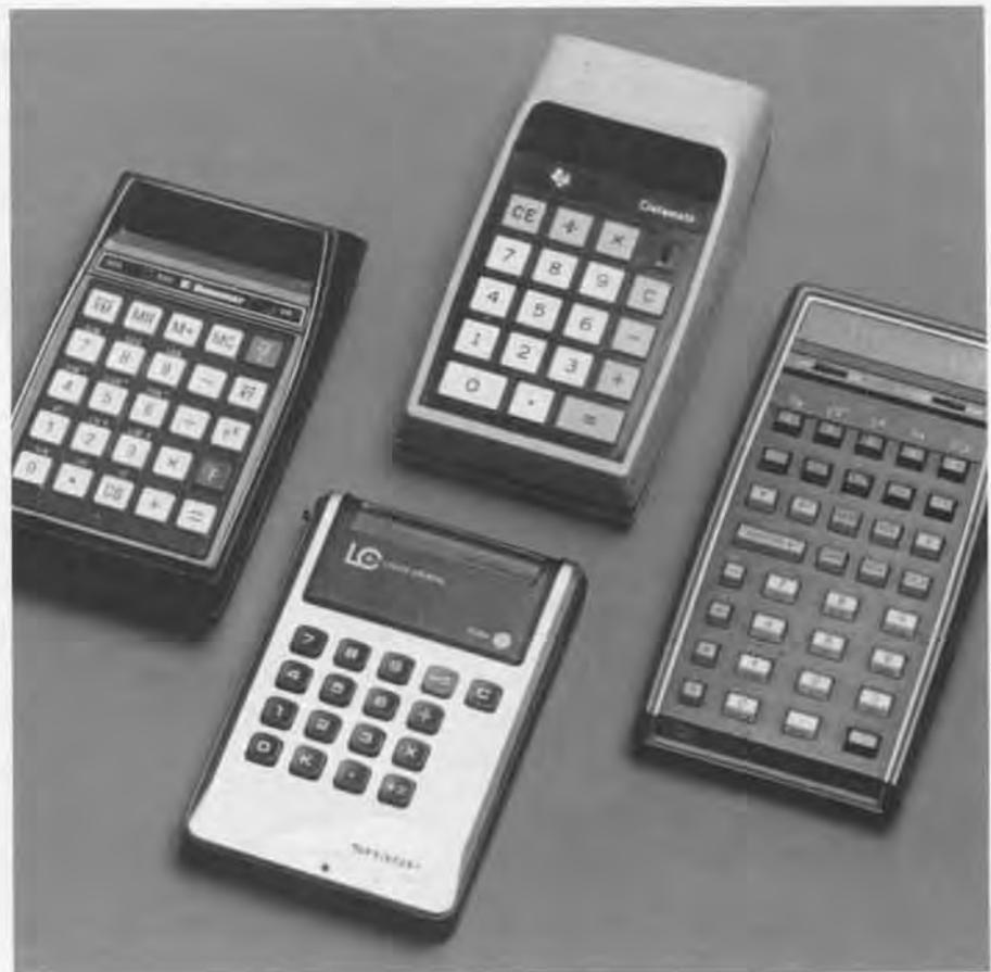
Early pocket calculators could only add, subtract, multiply, and divide. However, they offered speed and accuracy over most previous pocket calculators. The first electronic calculators were not cheap: the Bowmar 901B when introduced in 1971 sold for close to \$250. Within five years similar calculators sold for one-tenth as much, and far more powerful calculators were also available.
