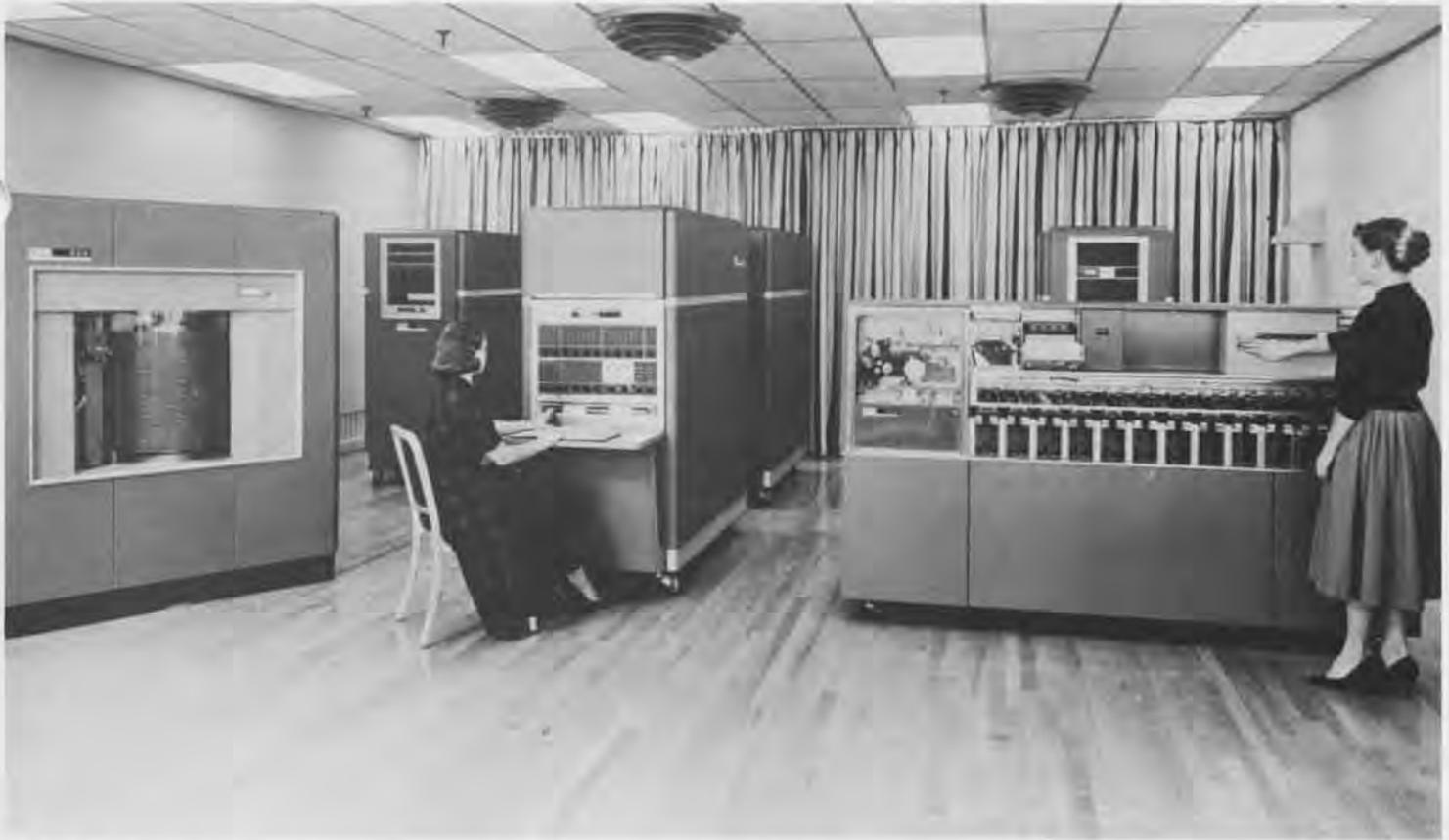
**IBM 650.** The IBM 650 was the most widely used first-generation computer. Hundreds were delivered between 1955 and 1959. Although the 650 was faster than other magnetic drum computers, its high success rate was a result of a well-integrated, punched-card input and output and its adaptability to existing punched-card systems.
