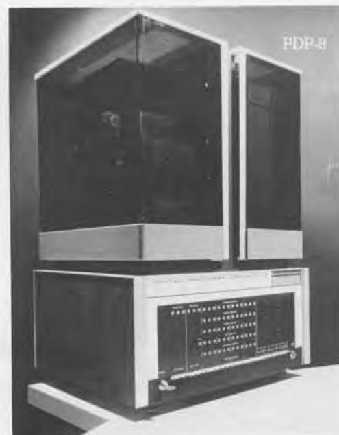
In April 1965, the idea of the minicomputer was realized with the delivery of the first PDP-8. The processor of this Classic Eight was housed in a transparent box revealing the elegance of its logic modules.
