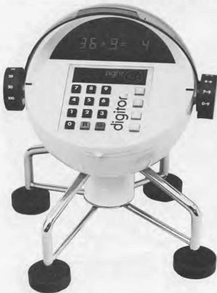
**Digitator, by Centurion Industries, 1974.** This is not a UFO or a highly advanced computer for space exploration. It is digitator, probably the first educational tool based on a microprocessor. Built around the Intel 4004 processor in 1974 digitator claimed to be a "flexible and challenging means of testing the arithmetic abilities of elementary school children." By adjusting the two side knobs the teacher or student can set the difficulty and length of a series of problems. Stu-
