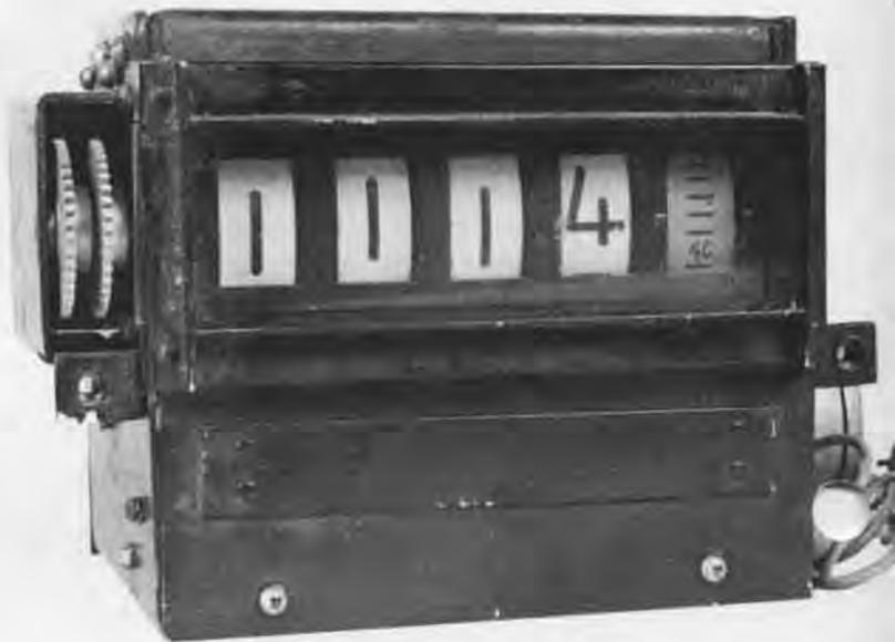
**BIZMAC Clock.** The BIZMAC was the result of an early attempt by RCA to produce a large-scale general-purpose computer for business applications. With its 29,000 tubes and 63,000 diodes, it was certainly one of the largest first generation computers ever built. The BIZMAC was one of the first commercial computers to use magnetic core memory. Later computers with full-scale core memories made BIZMAC obsolete.
