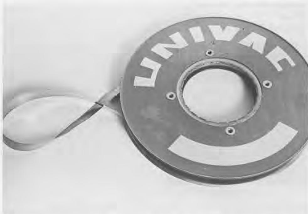
too, but it didn't look like a recording signal and I ignored it. John correctly interpreted it as a signal caused by improved magnetic properties due to the heat of soldering. His astute observations started me on a series of experiments on heat treating tape. It was not the final answer, but it was a key answer along the way.
