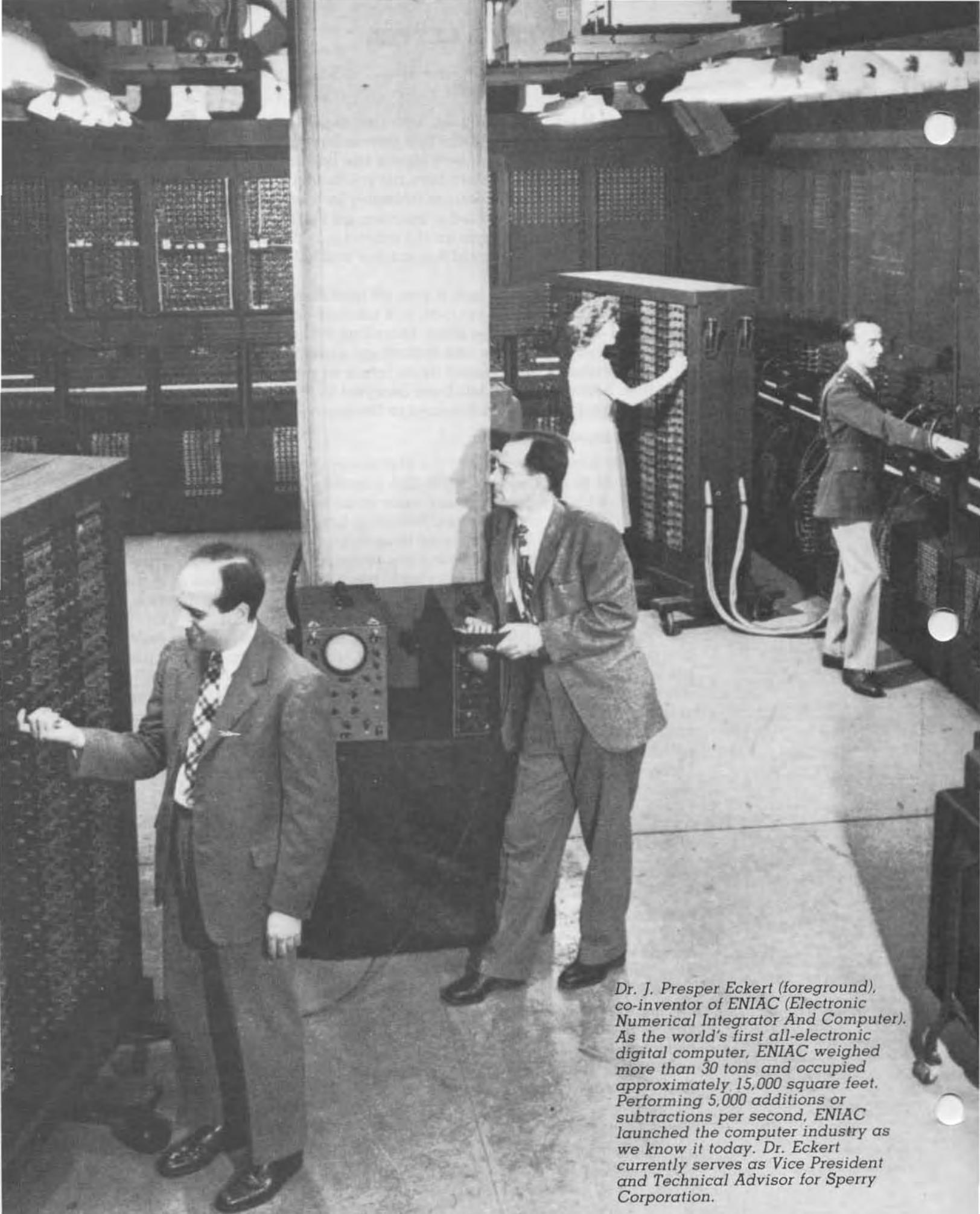
*Dr. J. Presper Eckert (foreground), co-inventor of ENIAC (Electronic Numerical Integrator And Computer). As the world's first all-electronic digital computer, ENIAC weighed more than 30 tons and occupied approximately 15,000 square feet. Performing 5,000 additions or subtractions per second, ENIAC launched the computer industry as we know it today. Dr. Eckert currently serves as Vice President and Technical Advisor for Sperry Corporation.*
