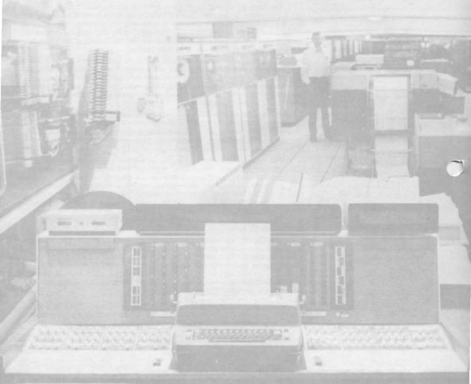
Project Stretch started in 1954 and introduced a number of new ideas evidenced by a set of new terminology such as "byte," "I/O interface," and the word "architecture" as applied to computers.
