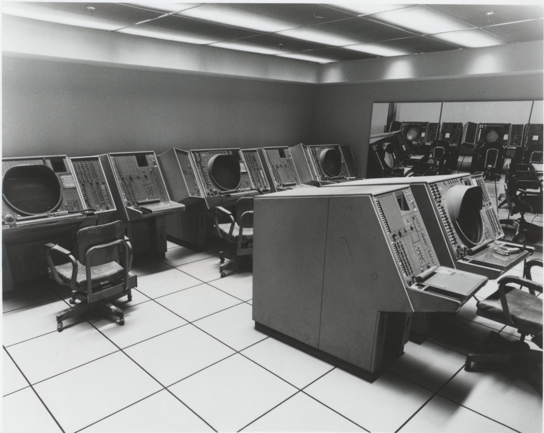
Pictured is "the Blue Room," the control room for the SAGE, the U.S. air defense system from 1958-1983. Here, Computer Museum visitors will see the oversized video display terminals that served as the first computer graphics output devices.
