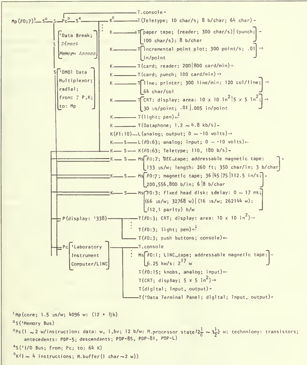
Fig. 1. DEC LINC-8-338 PMS diagram.
