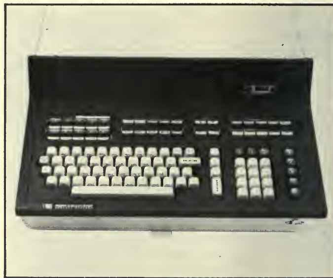
Fig. 6. Model 30 of the 9800 Series has an alphanumeric keyboard like a teleprinter. Its language is BASIC. It can be used as a desktop computer or a remote computer terminal, yet it maintains the convenience and user interaction of a programmable calculator.
