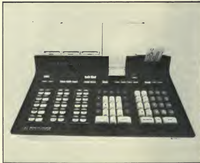
Fig. 2. Model 20 of the 9800 Series has a 16-character alphanumeric LED display that shows several keystrokes or program steps in context. Special features are a natural algebraic language, an interactive mode of operation, and plug-in modules that define the functions of the three lefthand keyblocks.
