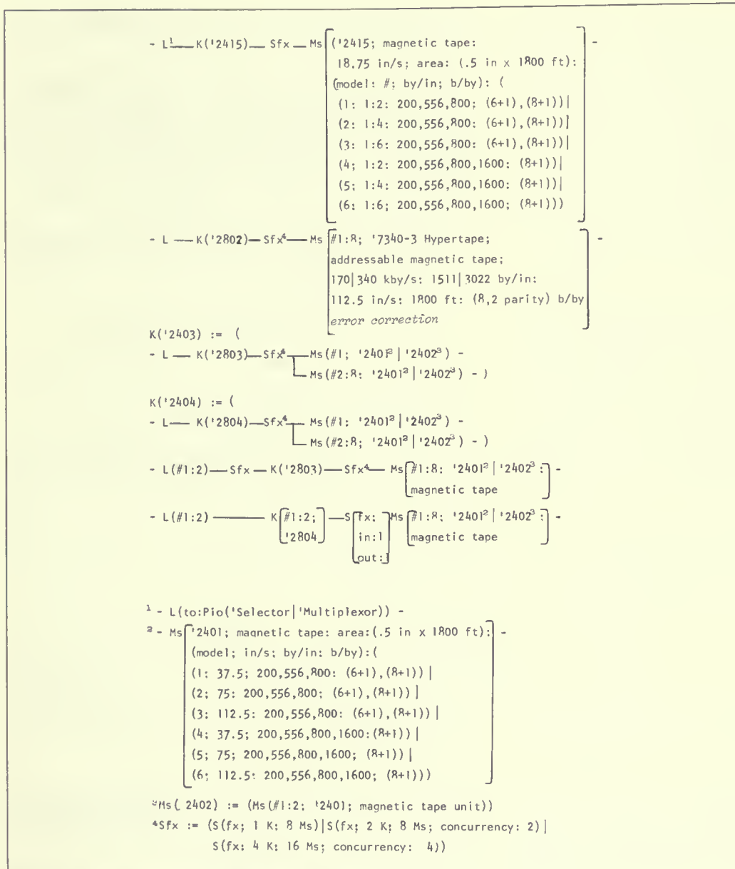
Fig. 13. IBM System/360 Ms(magnetic tape) PMS diagrams.
