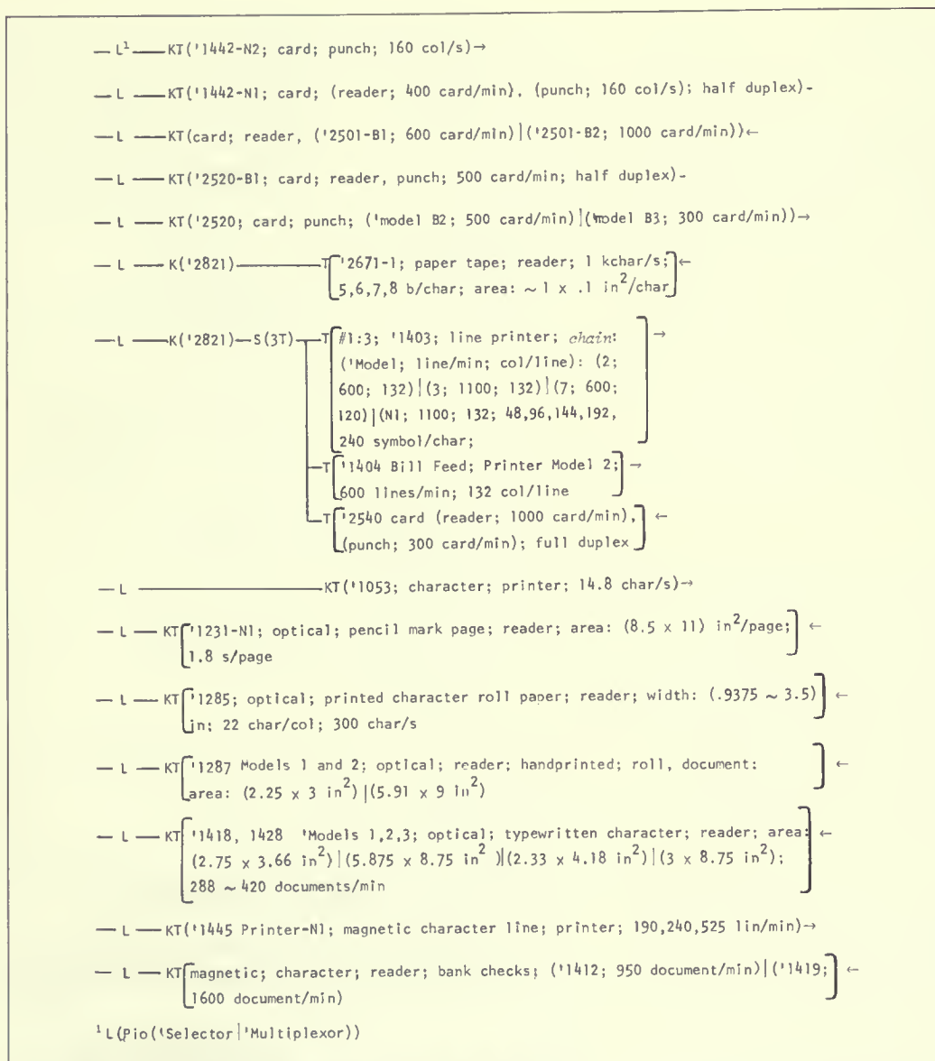
Fig. 15. IBM System/360 T(printer, reader, punch) PMS diagrams.
