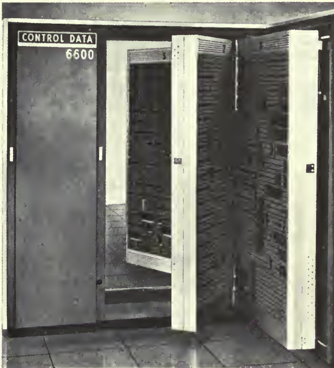
Fig. 9. 6600 main frame section.
