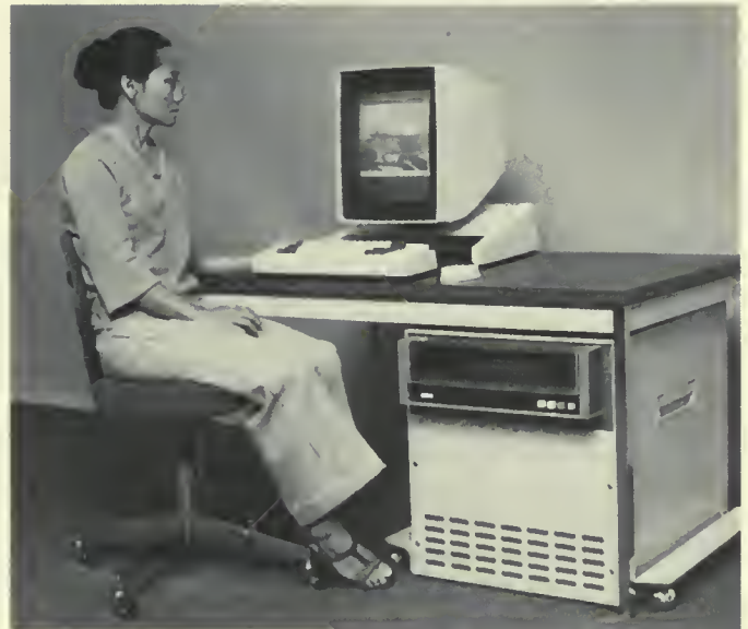
Fig. 1. The Alto personal computer, showing a user at work with the display, mouse, and keyset.
