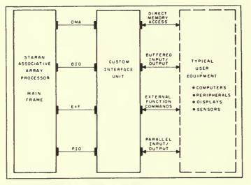
Fig. 1. STARAN system configuration.
