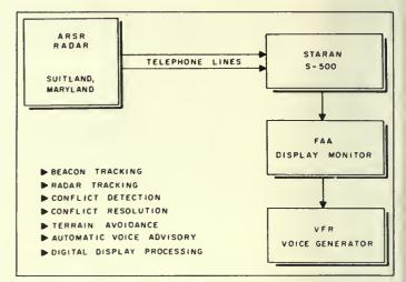
Fig. 9. Air traffic control application.
