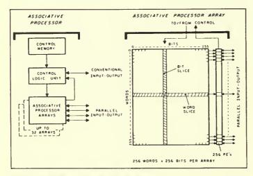
For many applications, the MDA memory is treated as a square array of bits, 256 words with 256 bits in each word. The bit-slice access mode (Fig. 2*a*) is used in the associative operations to access one bit of all words in parallel, while the word access mode (Fig. 2*b*) is used in the I/O operations to access several or all bits of one word in parallel.
