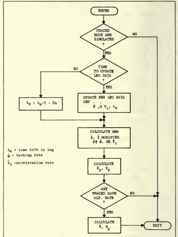
Fig. 12. Tracking simulation.
