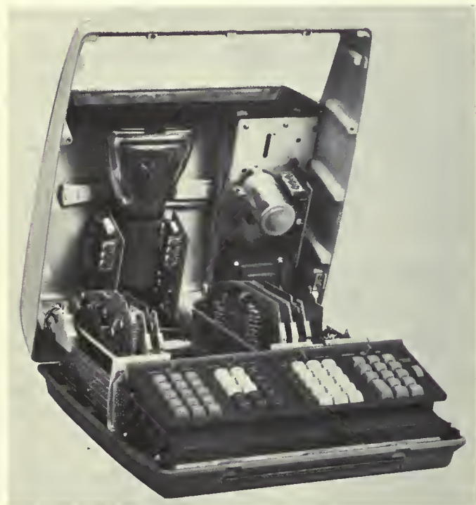
Fig. 14. Internal adjustments of the calculator are easily accessible by removing a few screws and lifting the top.
