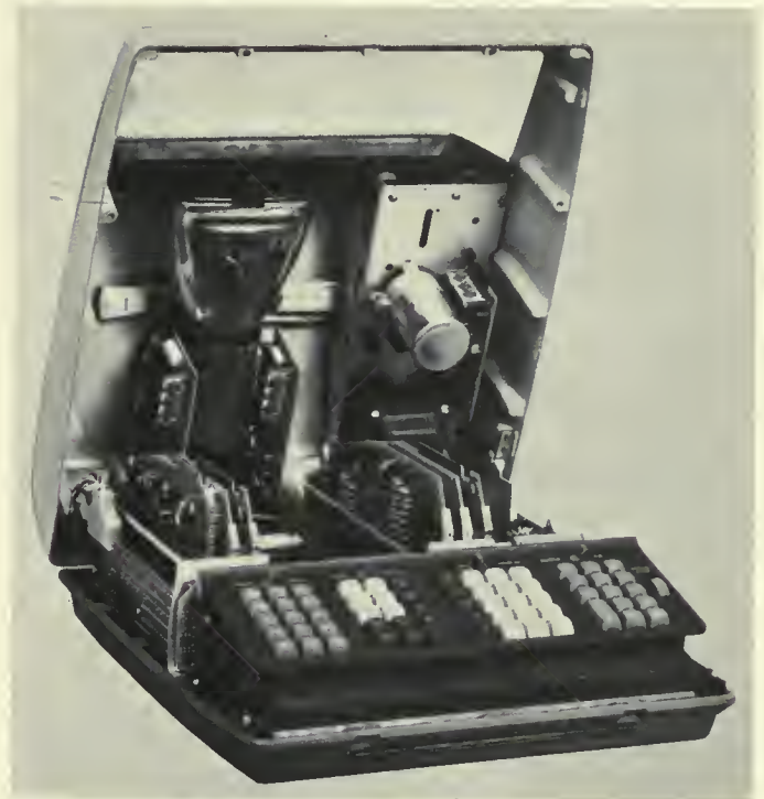
Fig. 14. international adjustments of the calculator are easily accessible by removing a few screws and lifting the top.
