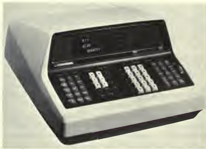
Fig. 1. This new HP Model 9100A calculator is self-contained and is capable of performing functions previously possible only with larger computers.
