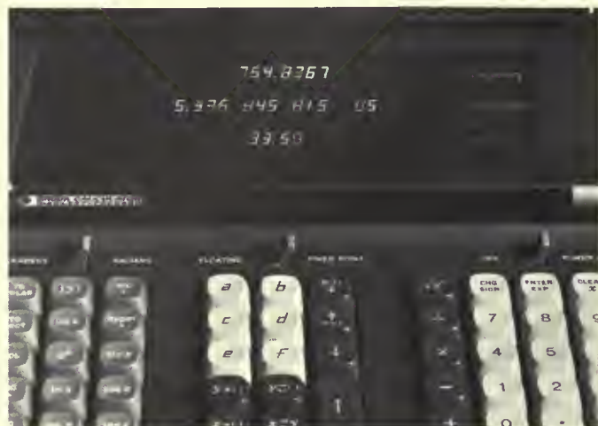
Fig. 2. Display in fixed point with the decimal wheel set at 5. The Y register has reverted to floating point because the number is too large to be properly displayed unless the digits called for by the DECIMAL-DIGITS setting are reduced.
