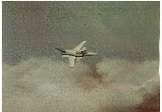
Fig. 12 Frame From X-29 Promotional Film. The X-29 aircraft is modeled by 40 quadric surfaces without texturing. The clouds are modeled by quadric surfaces with texturing.
