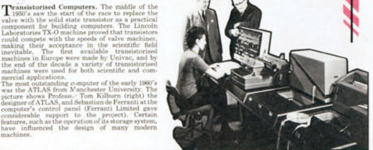
Transistorised Computers. The middle of the 1950s saw the start of the race to replace the valve with the solid state transistor as a practical component for building computers. The Lincoln Laboratories TX-0 machine proved that transistors could compete with the speeds of valve machines, making their acceptance in the scientific field inevitable. The first available transistorised machines in Europe were made by Univac, and by the end of the decade a variety of transistorised machines were used for both scientific and commercial applications. The most outstanding computer of the early 1960s was the ATLAS from Manchester University. The picture shows Professor Tom Kilburn (right) the designer of ATLAS, and Sebastian de Ferranti at the computer's control panel (Ferranti Limited gave considerable support to the project). Certain features, such as the operation of its storage system, have influenced the design of many modern machines.
