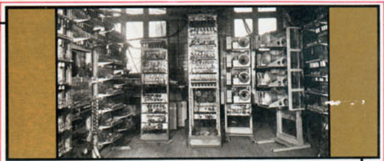
Valve Computers. The first practical stored program electronic computer to work anywhere in the world was the Cambridge University EDVAC (Electronic Delay Storage Automatic Calculator) in May 1948. Professor Maurice Wilkes designed this machine after visiting the Moore School of Electrical Engineering at the University of Pennsylvania the previous year. The Moore School had started work on the EDVAC computer earlier than Cambridge but its completion was delayed by the departure of Professors Eckert and Mauchly to form their own manufacturing company. The early machines used electronic valves and limited storage devices such as mercury delay lines, electrostatic and magnetic drum memories.
